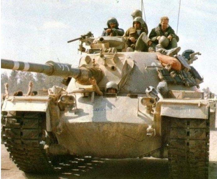
An Magach, Israeli designation for M48/60 based main battle tank, on its way to the front in 1973.
