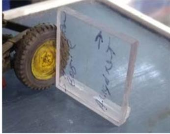
I can glue on a foot, and it will stand upright. The edge will be perpendicular to the build platform. I can also glue a cross piece on it and make a little T-square. I scratch a square line to make an alignment tool.
