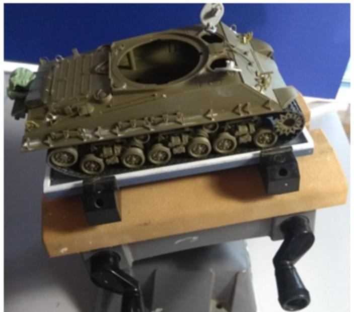
**Medium density fiberboard (MDF)** is manufactured so the top and bottom sides are flat and parallel. You can glue wet/dry sandpaper to scraps from the wood shop to create some very flat sanding tools. Each side is a different grit. You can wet sand with them, but if the edge gets wet, it will absorb water and
