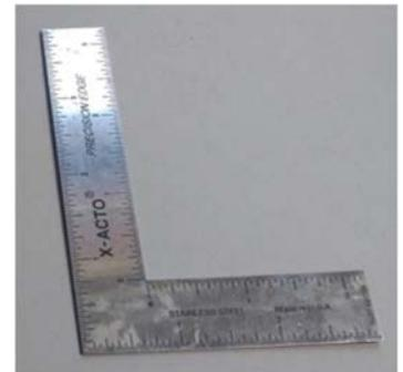
When using the metal square, I abut both the workpiece and the square to a straight piece of plastic so they are easier to keep aligned.
