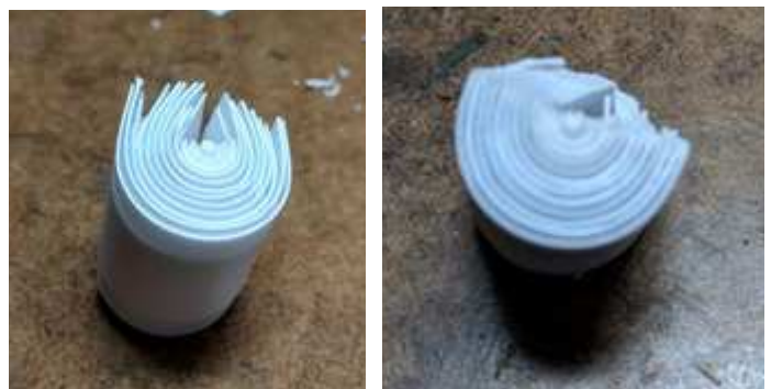
Left: Styrene sheet wrapping complete. Right: The wrapped sheet ends shaved down to form a half-pipe.
