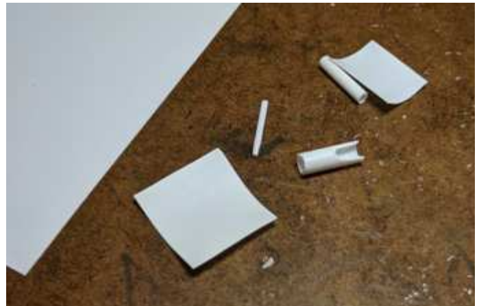
Initial styrene cut to form the inner core of the graining tool.
