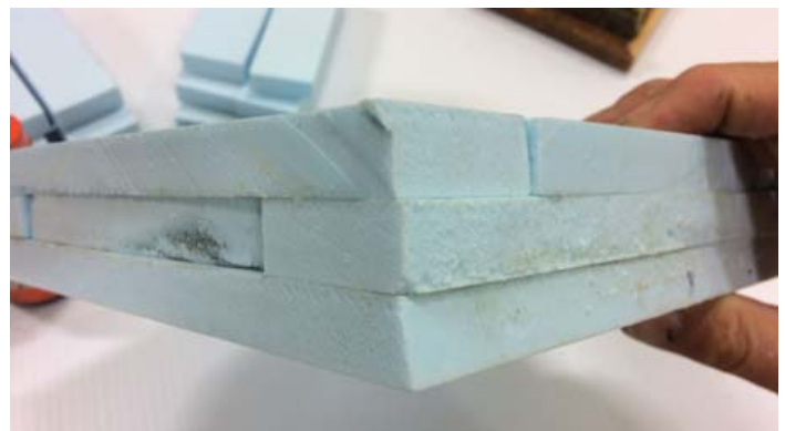
The overlay pattern as seen from the outside corner.
