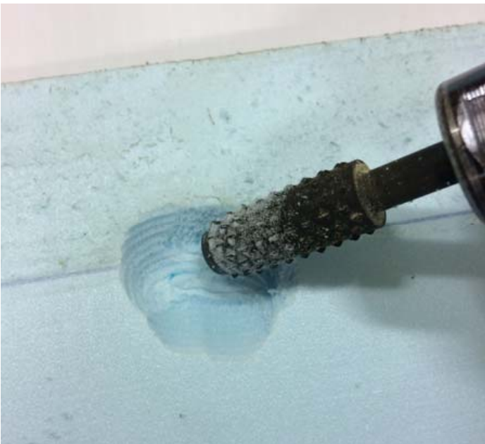
Forming the finger divots in the base. Remember not to go to deep!
