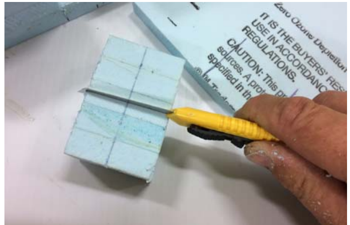
Cutting the tabs for the lid, using the material removed to form the access slot.
