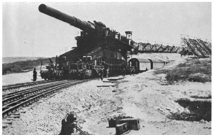
The German 80cm Schwerer Gustav Railway gun made its debut firing on fortifications and ammunition dumps inside Sevastopol.
