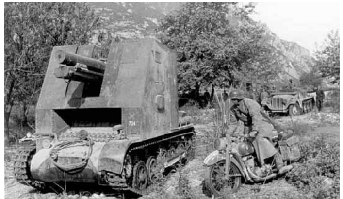
A German SIG 33, PzKpfw I mounting a 15cm infantry gun, supporting the invasion of Greece.
