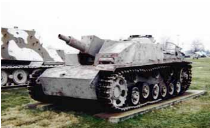
Stug. III Ausf. G with a 'short' barrel – blown off or cut off? . Suspension appears collapsed on this and the next photo.
