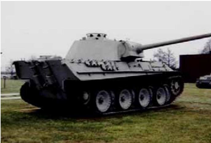
The later mantlet on the Panther G is evident with the added chin to aid in preventing shot deflection down through the top of the hull.
