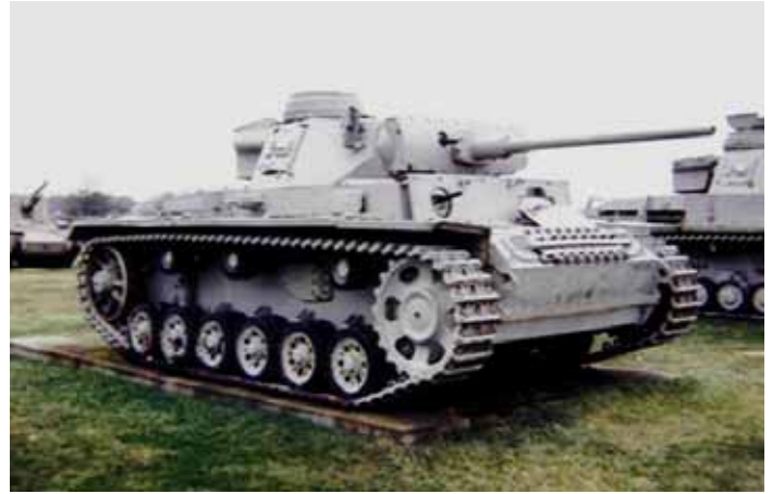
A better looking Panzer III Ausf. L. Had to get the books out to ID this one. No vision ports on the sides of the turret or on the right side of the mantlet.
