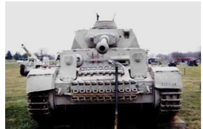
Hey, this one has two lengths of spare track links left. Odd that the transmission hatches were left open.
