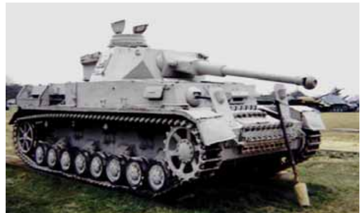
This Panzer IV appears to be an Ausf. F2 with long barreled gun and globular single baffle muzzle brake.
