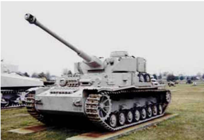
Probably a Panzer IV Ausf. H due to the long barreled gun and the side vision port for the driver.
